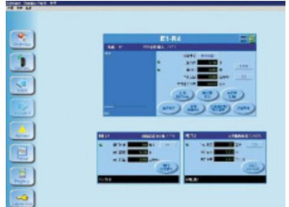
A Chinese language SCADAConnect interface provides operators at Fen River's control centre with real-time flow and water level information
