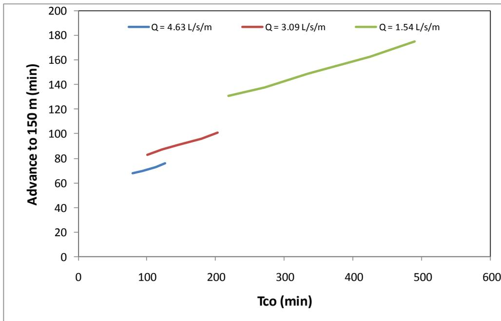
**Figure 3** Advance vs optimum  $T_{co}$  for summer pasture in a 400 m long bay on a cracking soil at various inflow rates
