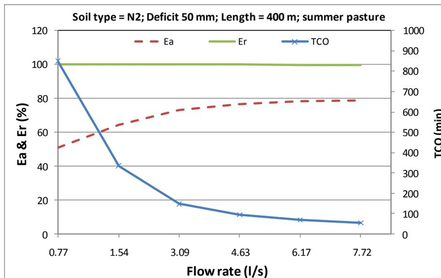
Figure 1 Example results for a moderately permeable non-cracking soil
