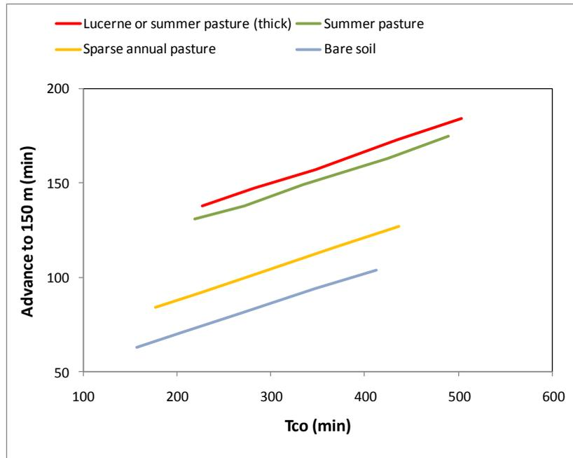
**Figure 2** Example of guidelines for selection of time to cut-off ( $T_{co}$ ) for a non-cracking soil type, bay length 400 m and flow rate 1.54 L/s/m
